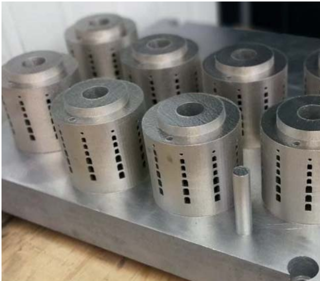
Additive Manufacturing: trim removed from the printing machine.
