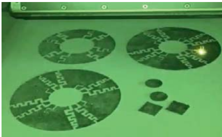
Additive Manufacturing: laser processing of Multistep-multipath trims.
